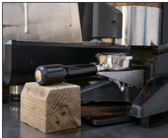
Figure 1: Wooden Block Used to Hold the Porta Filter
