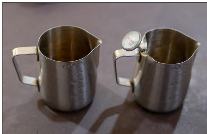
Figure 3: Pitcher with adapted thermometer
