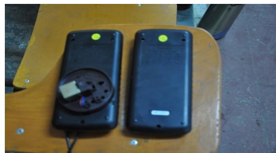
A voltmeter with an added sound system
